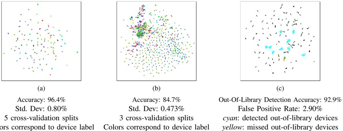
Fig. 1: Umap plots on 100 device classification, 500 device classification and 90/10 out-of-library detection tasks.
