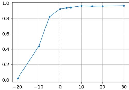
Fig. 3: 100 in-the-wild devices. Evaluation set accuracy as a function of SNR.
